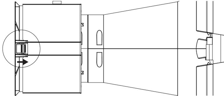
Step 2. Slide the lens tube down into the body until the locking lever can latch. Loosen focus lock knob and adjust focus as desired. Tighten to lock. Reverse process to remove.
