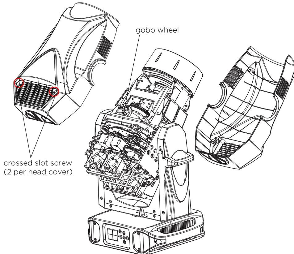
Step 3. If removing gobos via bottom of head assembly, undo fan tray assembly with thumb screw to access.
