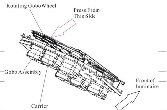
Step 5. Remove current gobo by carefully pressing on edges of gobo carrier with fingers, pressing gobo toward front end of luminaire (toward lens), and out of wheel.
