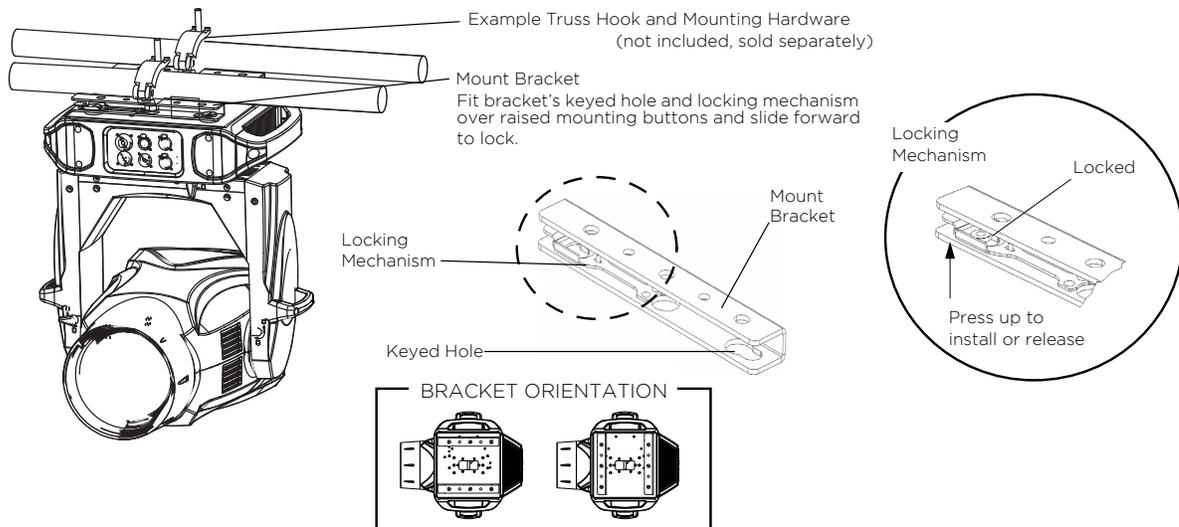
**Installing in Truss:**
