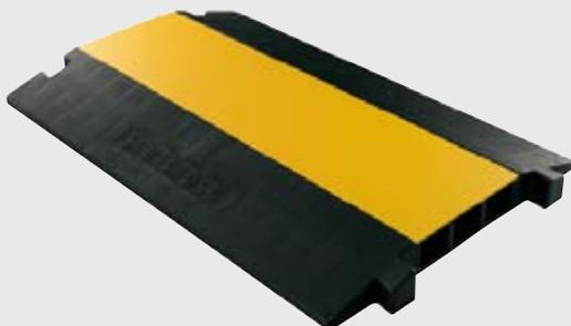
**CC30XT** This model is made of an injection-moulded rubber and polypropylene compound. It is suitable for protecting cables in areas where people and light vehicles cross. The top cover is made in pvc and fixed on the polyurethane base with 2 velcro strips.
