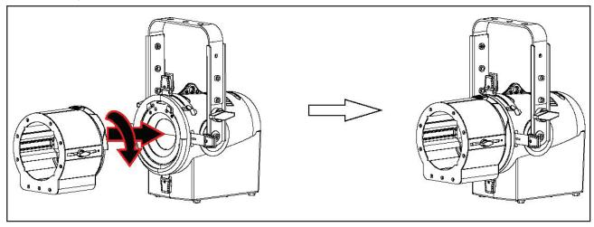
Step 2. Insert the lens tube into the adapter. After acheiving the desired beam edge, tighten the locking bolt.
