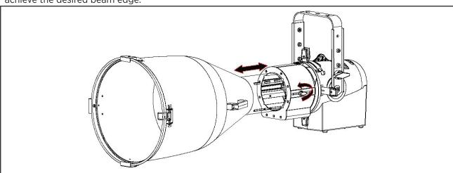
Step 2. Once the luminaire is focused, tighten the locking bolt.
