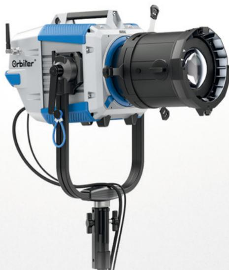
Two kinds of projection optics provide the desired output and quality. The projection optics contain high-end lenses to provide even illumination and color across the entire beam field for superior results. Fixed beam angles available are 15°, 25°, 35°. Wider angles might be added in future. The zoom projection optics allow for flexibility in all kinds of application.
