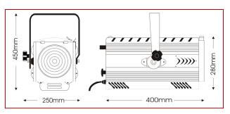
A high efficiency 230W led module featuring a PWM dimming power source harnessed in the high-specification optics of LDR fresnel spotlights.
