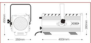
A high efficiency led module featuring a 380W tunable white COB power source harnessed in the high-specification optics of LDR fresnel spotlights.
