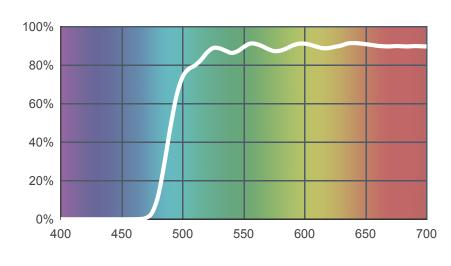
Light transmitted (Y%) for each colour wavelength (nm)
