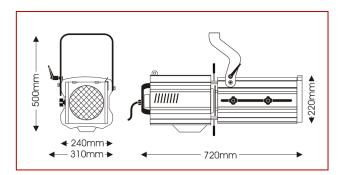
For closer projection in larger venues, this wide-angle 18° - 36° 2000W spotlight incorporates a zoom focus double condenser optical system, rotating gate, a cranked fork and a double microswitch interlock for safe lamp replacement.
