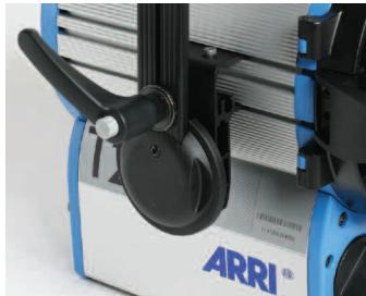
ARRI's new design creates a positive lock so there's no slippage when using heavy accessories. A stainless steel friction disc functions like a disc brake allowing the lamphead to be completely locked off with a minimum of force.
