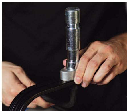
Before mounting the fixture, attach the proper mounting hardware to the stirrup. A spigot and spacer\* is included inside the box and should be attached with a 10mm hex or Allen wrench. The bolt must be fully tightened (50Nm of torque are adequate). Hanging models include a C-clamp instead of a spigot.
