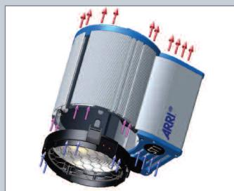
ARRI's cross cooling system moves a stream of air around the Fresnel lens and through the lamphead. In addition, air is channeled through the aluminum extrusion housing reducing lens temperature by 17% and housing temperatures by 25%. Cross cooling allows ARRI TRUE BLUES to safely operate at almost any tilt angle.
