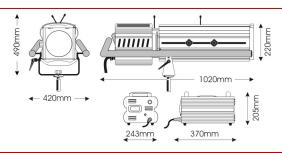
The Canto® 1200msr FF is an efficient, lightweight and extremely powerful followspot, ideal for all medium to long-throw applications. The MSR filling of the lamp guarantees pure, white light, whereas the short arc provides high beam intensity for professional entertainment lighting.
