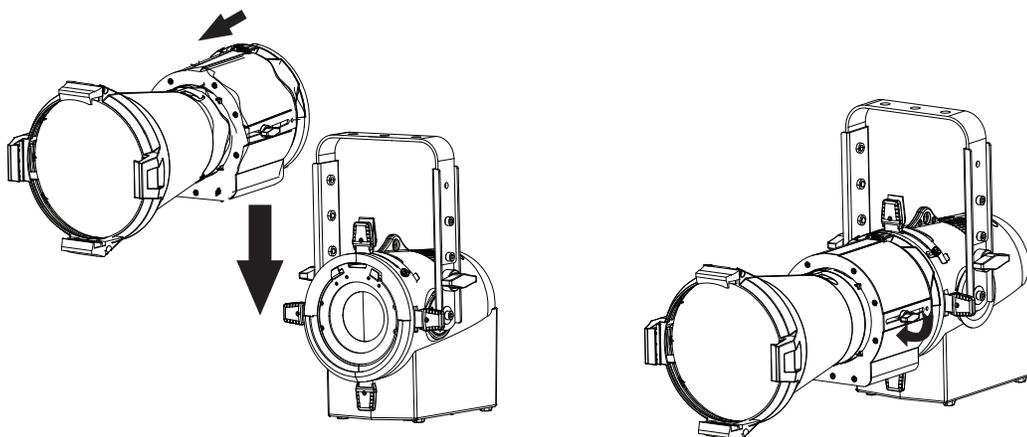
**NOTE:** Lens tube may need to be moved forward (away from the body) to install or remove. Loosen focus lock knob to adjust.
