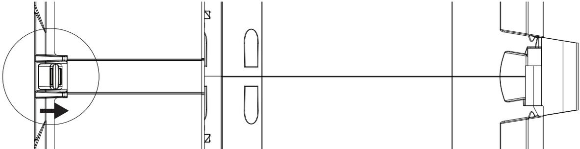
Step 2. Slide the lens tube down into the body until the locking lever can latch. Loosen focus lock knob and adjust focus as desired. Tighten to lock. Reverse process to remove.
